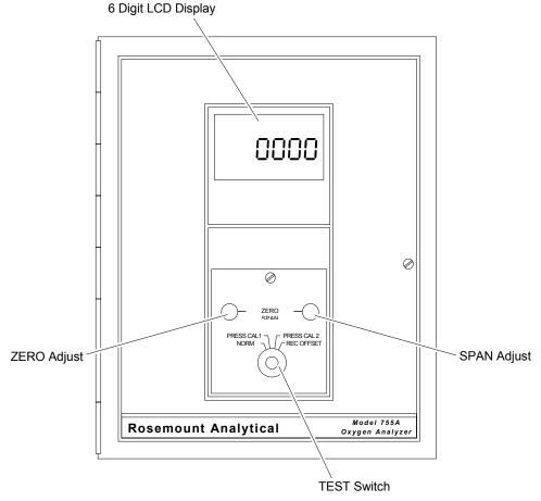
Figure 1-1. Model 755A Oxygen Analyzer
